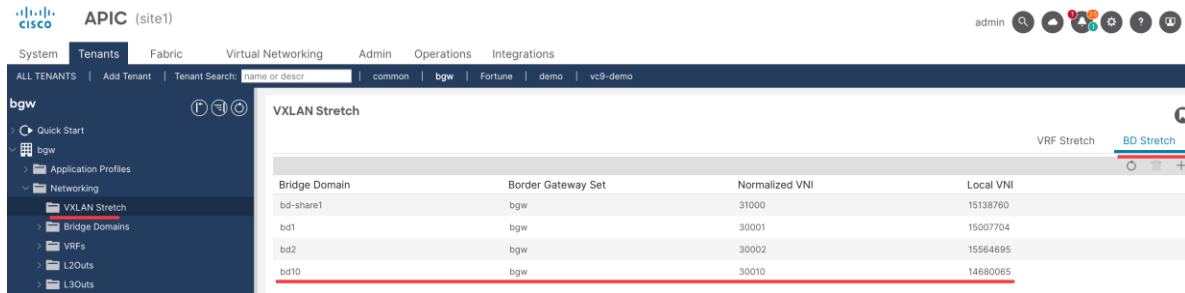
Figure 134. ACI Site 1 deploy bd10 on border gateway
