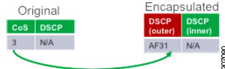
Figure 3: Copy of Priority from Layer-2 Frame to VXLAN Outer Header
