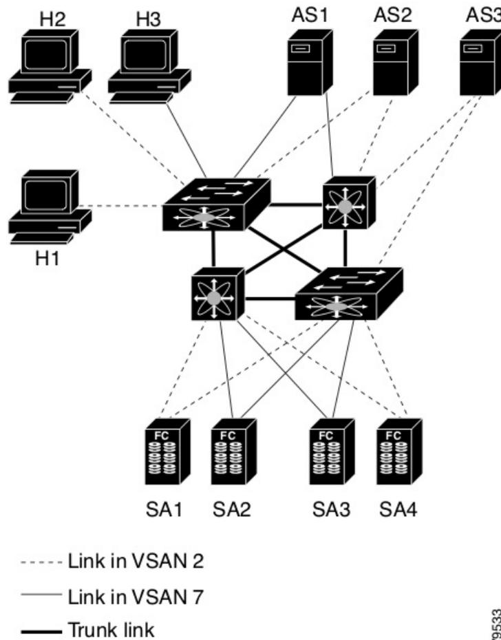
The four switches in this network are interconnected by VSAN trunk links that carry both VSAN 2 and VSAN 7 traffic. You can configure a different inter-switch topology for each VSAN. In the preceding figure, the inter-switch topology is identical for VSAN 2 and VSAN 7.
