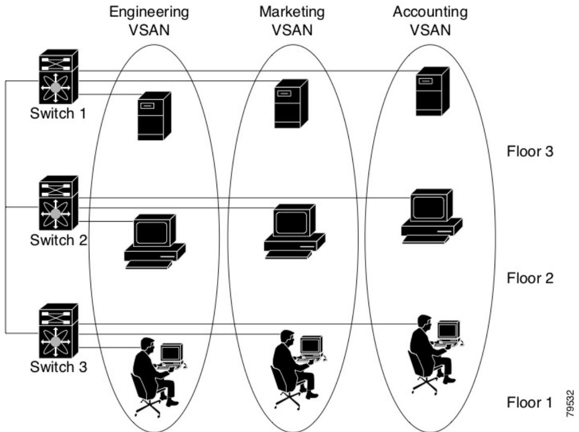
The application servers or storage arrays can be connected to the switch using Fibre Channel or virtual Fibre Channel interfaces. A VSAN can include a mixture of Fibre Channel and virtual Fibre Channel interfaces.
