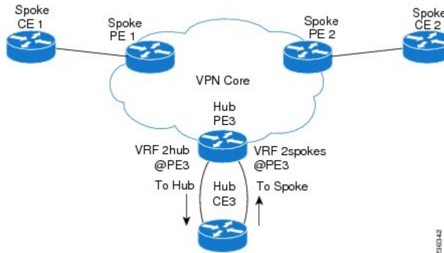
As shown in the figure, a hub-and-spoke topology is typically set up with a hub PE that is configured with two VRFs:
