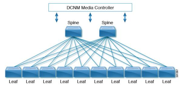
Media sources and receivers connect to the leaf switches, and receivers initiate IGMP join requests to the leaf switches in order to receive the media traffic.
