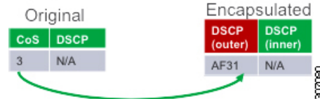
Figure 3: Copy of Priority from Layer-2 Frame to VXLAN Outer Header
