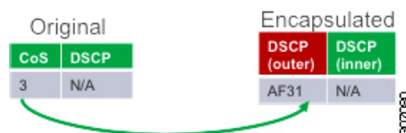
Figure 38: Copy of Priority from Layer-2 Frame to VXLAN Outer Header
