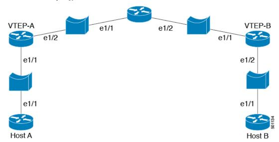
This topology can simulate basic vxlan functionality on Cisco Nexus 9000v platform. Similar bridge/vSwitch setup should be done as shown in other topology examples.
