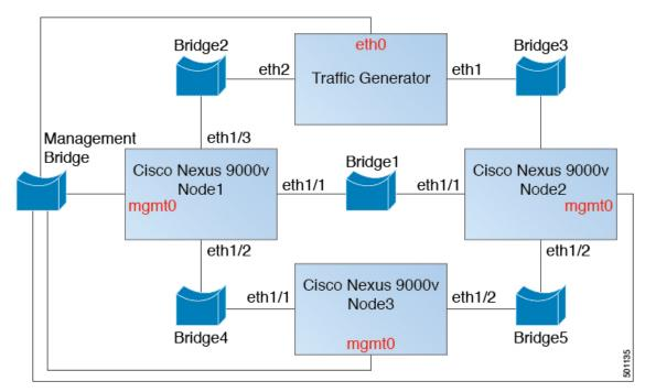
The nodes in the above diagram are instantiated using the hypervisor specific machine definitions. For networking, each data port interface pair needs to be connected to unique bridge/vSwitch. All the management ports of the Cisco Nexus 9000v (mgmt0) need to be connected to the management bridge and provided a unique IP address, which will enable access to these devices from an external network.
