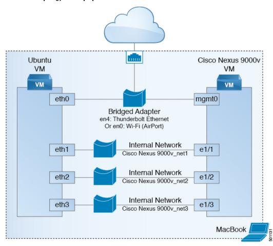
An example diagram above is a typical configuration with Cisco Nexus 9000v and Ubuntu VM two node system. In this case, Both Ubuntu VM and Cisco Nexus 9000v would obtain IPs statically or dynamically visa DHCP protocol reachable from cloud. Similarly, both Ubuntu and Cisco Nexus 9000v can be managed through management network. Ubuntu VM can send/receive packets to Cisco Nexus 9000v through Cisco Nexus 9000v data ports, eth1/1, eth1/2, and eth1/3, or ... e1/9.
