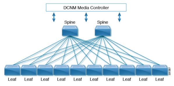
Media sources and receivers connect to the leaf switches, and receivers initiate IGMP join requests to the leaf switches in order to receive the media traffic.
