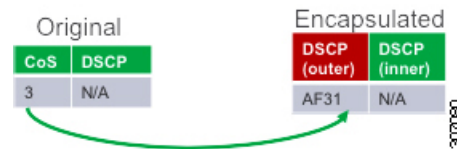
Figure 3: Copy of Priority from Layer-2 Frame to VXLAN Outer Header
