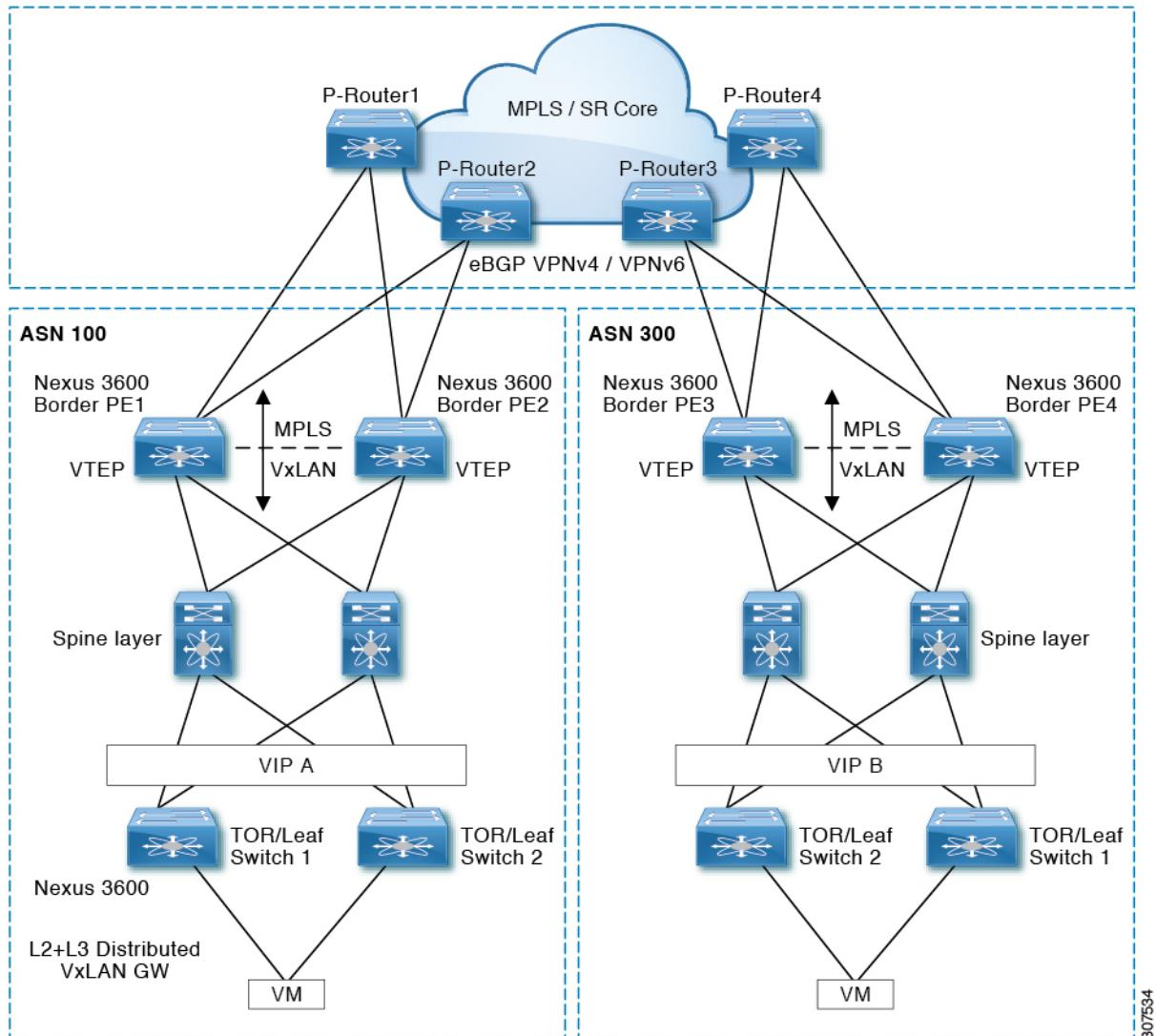
In the previous diagram, two DC pods, each running VXLAN, are being Layer 3 extended over a WAN/Core running MPLS/SR. Another method is classical MPLS L3VPN using LDP. The edge devices in the DC domain (border PE1, PE2, PE3, and PE4) are the DCI nodes doing the handoff between VXLAN and the MPLS-based Core network.
