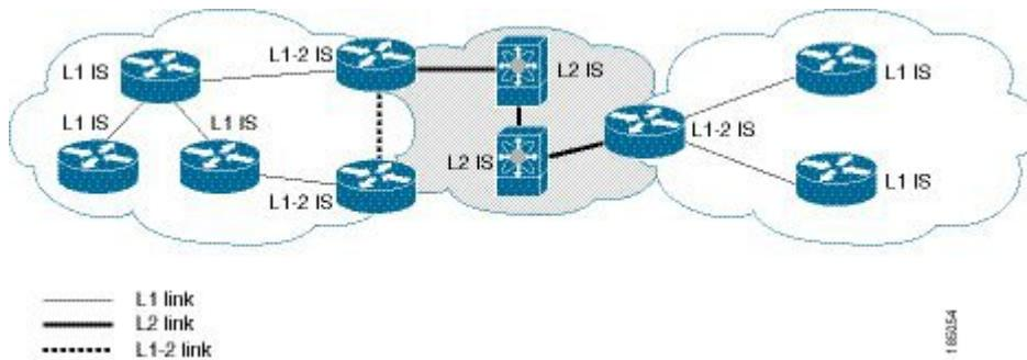
An autonomous system boundary router (ASBR) advertises external destinations throughout the IS-IS autonomous system. External routes are the routes redistributed into IS-IS from any other protocol.
