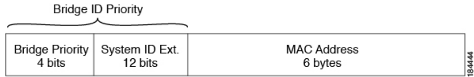
Figure 1: Bridge ID with Extended System ID
