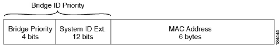
Figure 1: Bridge ID with Extended System ID
