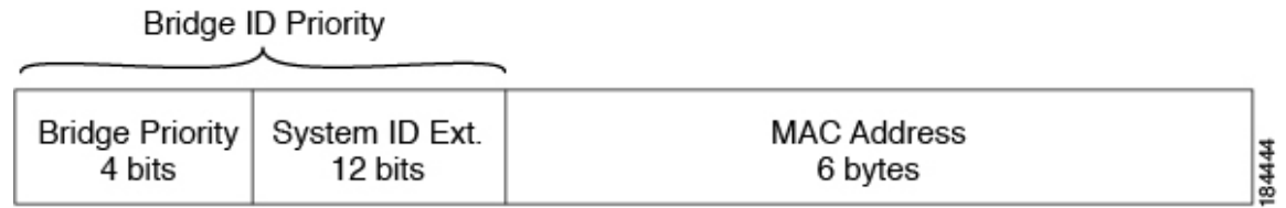
Figure 6: Bridge ID with Extended System ID
