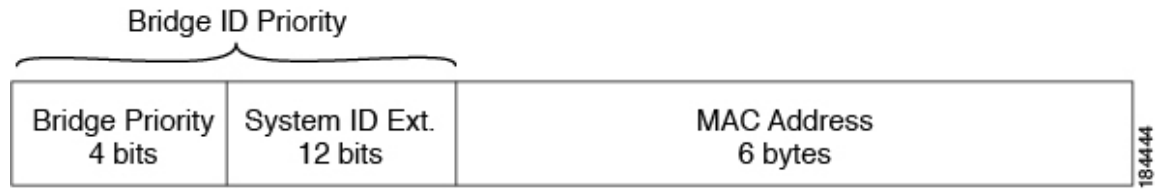
Figure 6: Bridge ID with Extended System ID
