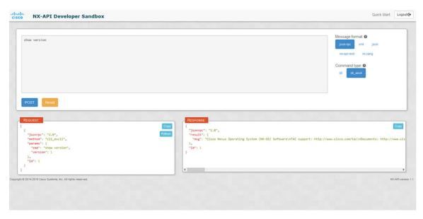
Controls in the Command pane allow you to choose a message format for a supported API, such as NX-API REST, and a command type, such as XML or JSON. The available command type options vary depending on the selected message format.
