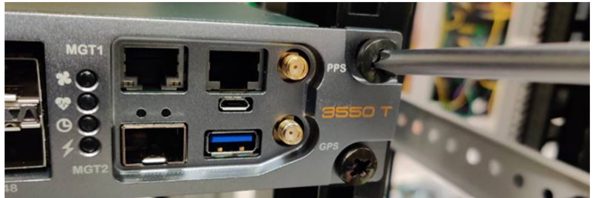
Figure 3: Fasten the Nexus 3550-T in the normal manner.
