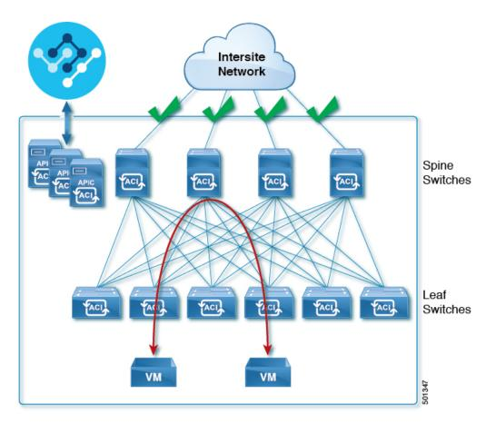
You can choose to mix spine switches supported by Multi-Site with switches that are not supported within the same Cisco APIC fabric, but only the supported switches can connect to the intersite network as shown in the following figure.
