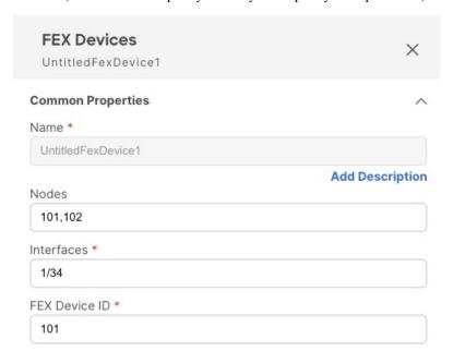
The above configuration means that there are two FEX devices, one connected to leaf switch 101 and another connected to leaf switch 102 with both devices having FEX ID 101. Since FEX ID is limited to the leaf switch scope, FEX devices that are connected to different leaf switches can have the same IDs.
