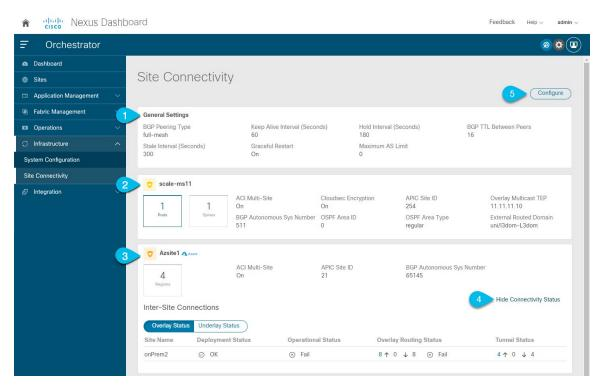
1. The **General Settings** tile displays information about BGP peering type and its configuration. This is described in detail in the next section.
