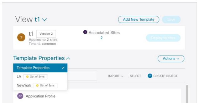
• Select the template and click **Deploy to sites** to bring up the configuration comparison screen to check which objects contain configuration drifts:
