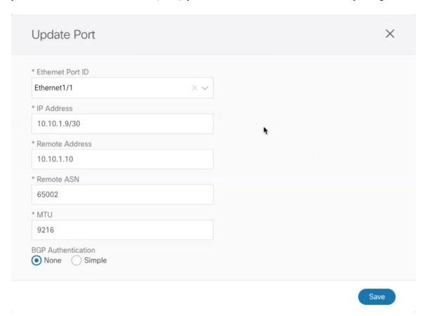
Provide the following information specific to your deployment for the port that connects this border gateway to a core switch or another border gateway:
