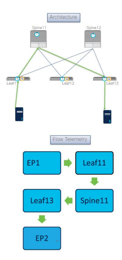
The Flow Telemetry line crossing every switch in the illustration represents the switches that are capable of exporting the Flow Telemetry data. For Example: With two flow telemetry HOP lines, the packet flows from Leaf 1.1 to Spine 1.1 and then to Leaf 1.3. This is considered as 3-Hop Flow Telemetry.
