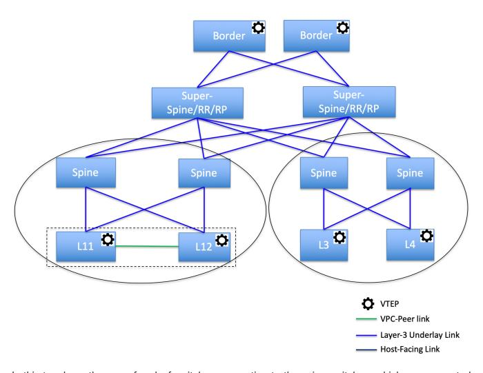
In this topology, there are four leaf switches connecting to the spine switches, which are connected to two super spine switches. These super spine switches are connected to the border or border gateway leaf switches.
