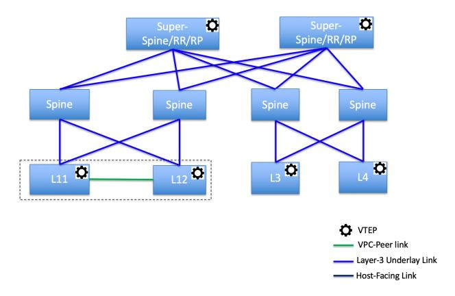
In this topology, leaf switches are connected to spines, and spines are connected to super spine switches which can be super spines, border super spines, and border gateway super spines.
