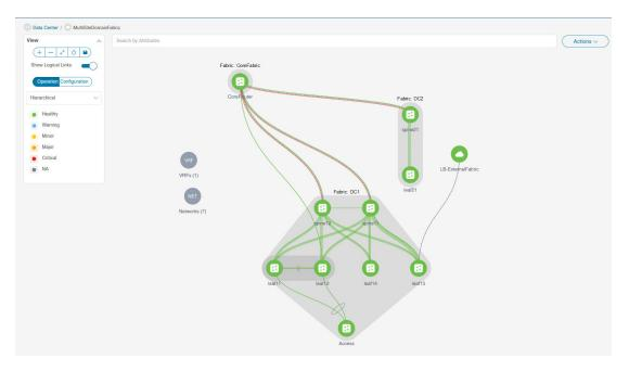
• **Member fabric topology view** – A member fabric and its switches are displayed. In addition, the connected external fabric is displayed.
