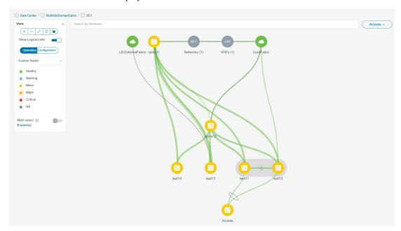
• A boundary defines a standalone VXLAN fabric, and each member fabric in the MSD\_Fabric fabric. A fabric's devices are confined to the fabric boundary. You can move a switch icon by dragging it. For a better user experience, in addition to switches, NDFC allows you to move an entire fabric. To move a fabric, place the cursor within the fabric boundary (but not on a switch icon), and drag it in the desired direction.
