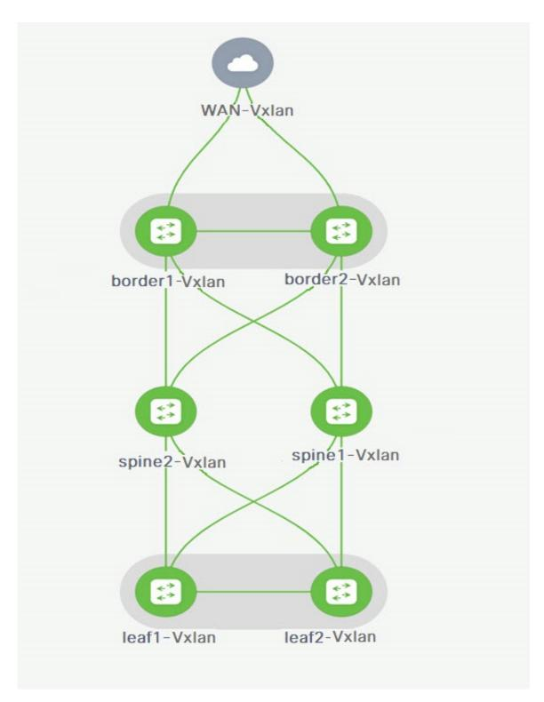
In this example, you can enable VRF Lite connections between DC-Vxlan Border leaf and WAN-Vxlan Edge router.
