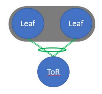
• ToR switches with port channels connected to leaf switches individually. The leaf switches are in a vPC pair.
