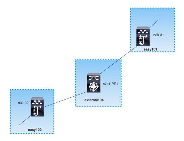
This topology shows only the border devices in the Easy Fabric and the core or edge router in the External Connectivity Network fabric.
