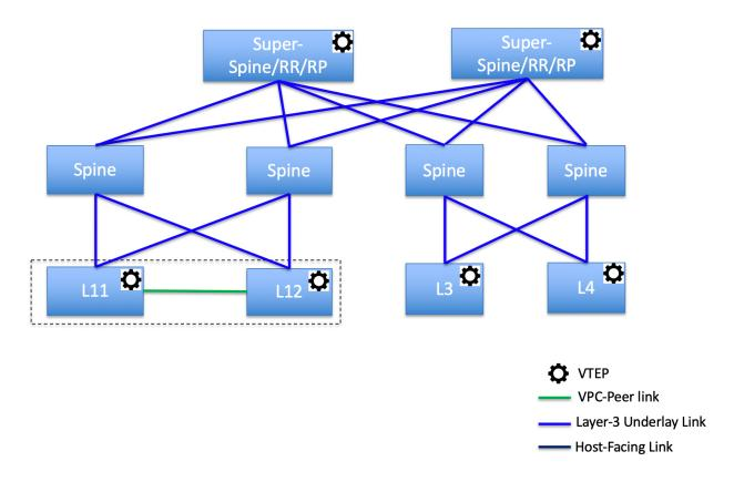
In this topology, leaf switches are connected to spines, and spines are connected to super spine switches which can be super spines, border super spines, and border gateway super spines.
