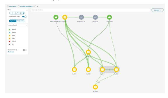
• A boundary defines a standalone VXLAN fabric, and each member fabric in the VXLAN EVPN Multi-Site fabric. A fabric's devices are confined to the fabric boundary. You can move a switch icon by dragging it. For a better user experience, in addition to switches, NDFC allows you to move an entire fabric. To move a fabric, place the cursor within the fabric boundary (but not on a switch icon), and drag it in the desired direction.
