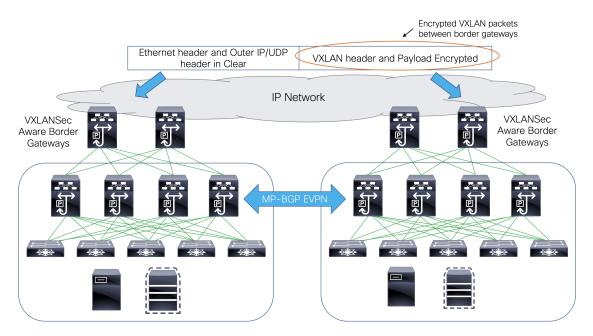
CloudSec feature is supported on Cisco Nexus 9000 Series FX2 platform with Cisco NX-OS Release 9.3(5) or later. The border gateways, border gateway spines, and border gateway superspines that are FX2 platforms, and run Cisco NX-OS Release 9.3(5) or later are referred as CloudSec capable switches.
