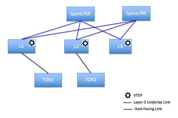
The following topology with ToR switches is not supported in NDFC:
