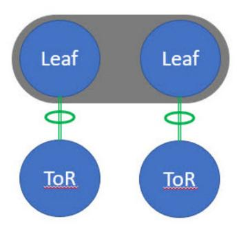
• ToR switches with back-to-back vPC connections. The leaf switches and ToR switches are both in vPC pairs.
