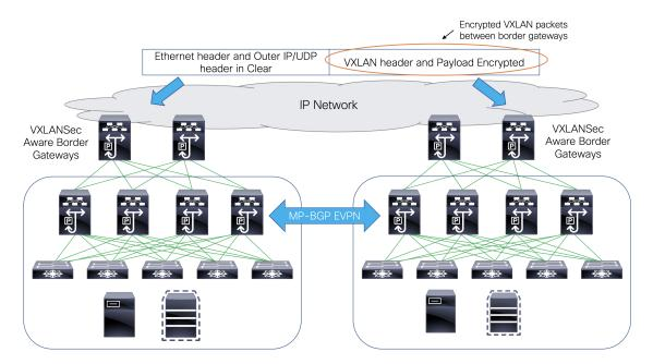
CloudSec feature is supported on Cisco Nexus 9000 Series FX2 platform with Cisco NX-OS Release 9.3(5) or later. The border gateways, border gateway spines, and border gateway superspines that are FX2 platforms, and run Cisco NX-OS Release 9.3(5) or later are referred as CloudSec capable switches.
