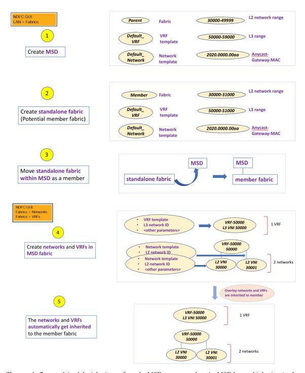
The sample flow explained the inheritance from the MSD to one member. An MSD has multiple sites (and hence, multiple member fabrics under an MSD). A sample flow from an MSD to multiple members:
