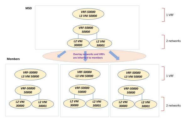
In this example, VRF-50000 (and L3 network with ID 50000), and L2 networks with IDs 30000 and 30001 are created in one go. Networks and VRFs are deployed on the member fabric switches, one after another, as depicted in the image.
