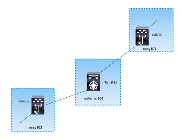
This topology shows only the border devices in the Data Center VXLAN EVPN and the core or edge router in the External Connectivity Network fabric.
