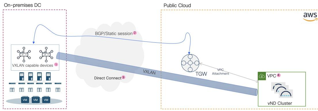
① On-premises device with VXLAN support for example, Catalyst 8000 series router, Nexus 9000
