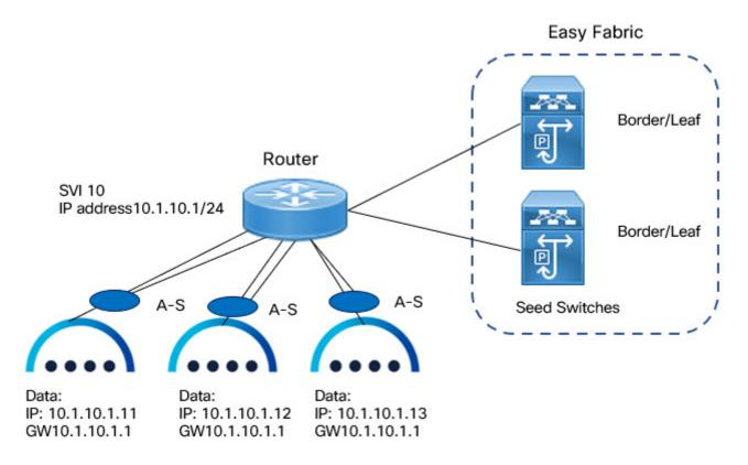
If you want POAP Layer-3 adjacency to the switches, you must add the Nexus Dashboard node IP address as DHCP Relay address:
