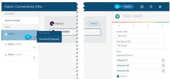
a) In the top right of the **Fabric Connectivity Infra** screen, choose the appropriate **Deploy** option to deploy the configuration.
