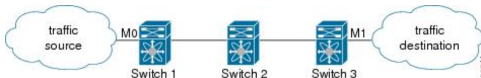
Figure 8: Denying Traffic on the Inbound Interface
