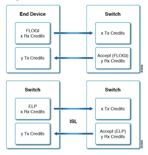
Each buffer location holds exactly one Fibre Channel frame regardless of size. As a frame is to be transmitted, the sender checks the remaining Tx BB\_credit number. If it is greater than 0, a frame can be transmitted. The sender then decrements Tx BB\_credit remaining number and transmits the frame. After the frame is received
