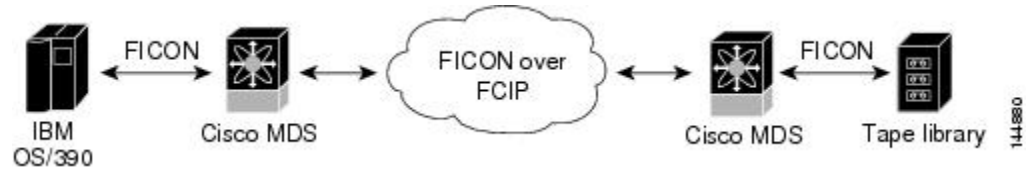
Figure 60: Host Accessing Standalone IBM-VTS (Virtual Tape Server)/STK-VSM (Virtual Shared Memory)
