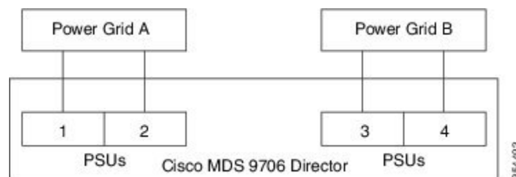
Figure 26: Cisco MDS 9706 Grid-PSU Connections
