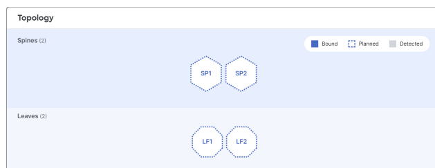
Figure 7: Spine and leaf fabric with 2 spine switches and 2 leaf switches
