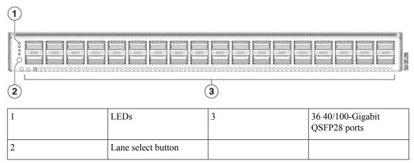
To determine which transceivers, adapters, and cables are support this switch, see the Cisco Transceiver Modules Compatibility Information document.
