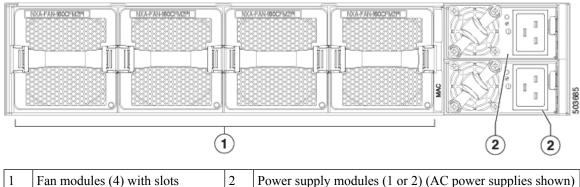
Fan modules (4) with slots numbered from 1 (left) to 4 (right)
