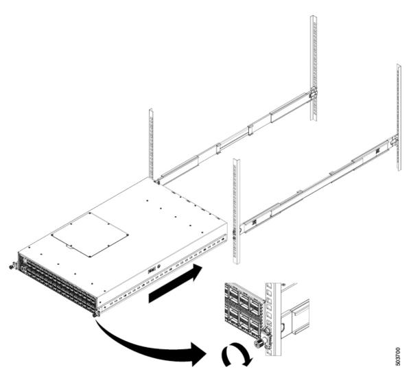
Step 7 If installing from the back of the rack, slide the chassis into the rack by aligning the inner rails into the outer rails, and sliding the chassis forward until the front panel is flush with the front of the rack. Then slide the retainer screws out to align with the rack and then secure the thumb-screws on the inner rails into the rack, as shown in the following illustration:
