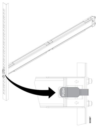
**Step 4** Install the two outer rails to the back posts of the rack by extending them into place, as shown in the following illustration:
