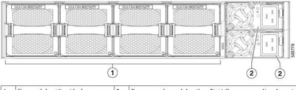
Fan modules (4) with slots numbered from 1 (left) to 4 (right)
