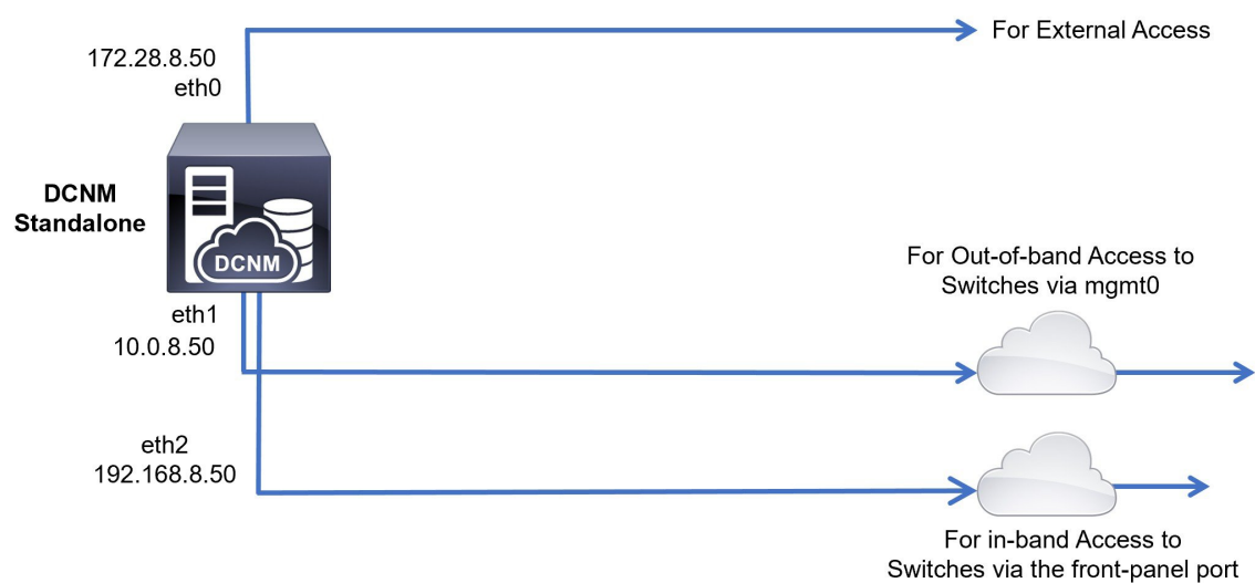
Figure 11: Cisco DCNM Standalone Deployment without Compute Cluster
