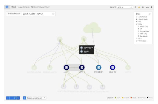
The traffic from **Source** traverses to the service leaf where the firewall is configured. Based on firewall rules, traffic is allowed to reach the destination, Leaf 15.
