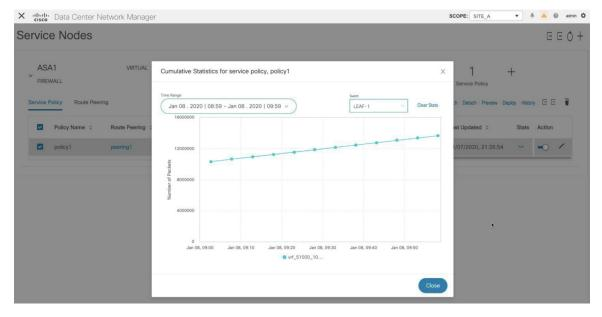
Statistics are displayed for forwarding traffic on the source switch, for reversed traffic on the destination switch, and for traffic in both directions on the service switch.
