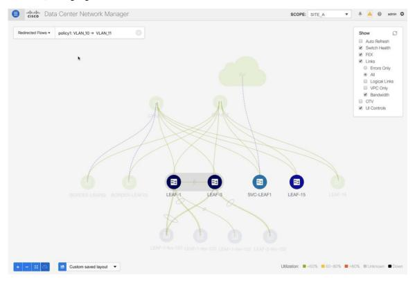
**Step 4** The service node is shown as connected by a dotted line to the leaf switch on the topology window. Hover over the dotted line to get more information about the interface.
